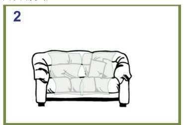
At time of final packing for a three seated sofa, the seat and back area should be covered with two pieces of 160cm x 60cm Micro-Pak® Sheet.
