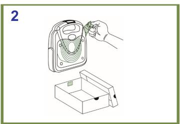
At time of final packing, one piece of Micro-Pak® Sticker should be placed on the upper short side of box base opposite to the hole.
