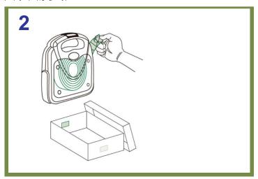
At time of final packing, two pieces of Micro-Pak® Sticker should be placed at each short end of the box.
